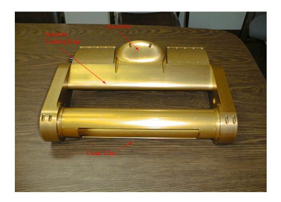
Figure 22. Extinctiometer Sample Head
