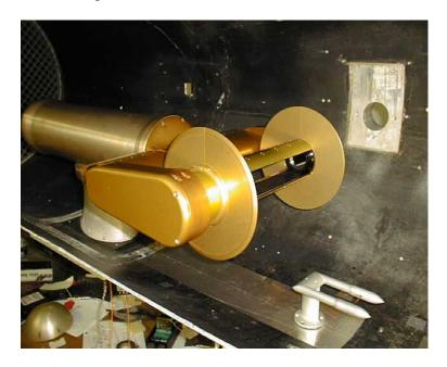
**Figure 38.** Extinctiometer sample head in wet wind tunnel during second round of tests with turbulence fences installed.
