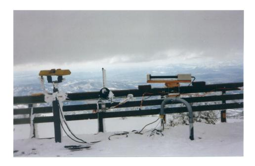
**Figure 2.** The SPEC automatic cloud spectrometer (ACS)(left) and the cloud extinctiometer (right) mounted on a rail on the roof of Storm Peak Observatory.
