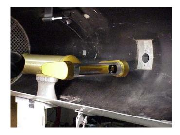
**Figure 36.** Extinctiometer sample head in wet wind tunnel during first round of tests.
