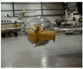
Figure 41. Side and head on views of transmissometer retroreflector shroud.
